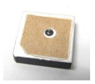
Note: Picture shown here is for reference. Actual antenna is only 2mm thick.
